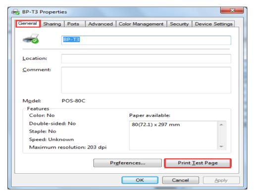
The drive has been installed successfully when test page is printed.
