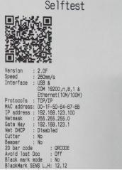
2. After confirming the IP, then connect to the computer(connect the computer with printer through Switch or Network cable, remark: if connect through Router, maybe can not modify) After connecting, amending through the testing software which in our CD, as below:
