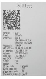
If selftest note same as the above picture, it means modifying successful, this method is suitable for all Lan port printers. For 3 in 1 port printers, 2 other modifying methods can be used as follows:
